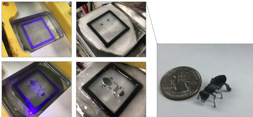
Fig. 13. The building process and result of the 3D ant.
